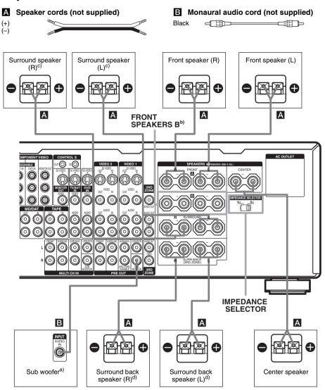
a) When you connect a sub woofer with an auto standby function, turn off the function when watching movies.
